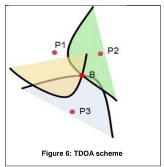
As shown in Figure 6 a tagged object (B) transmits a message that is received by all the readers (P1, P2 and P3 in the diagram shown here). Because radio waves travel at a constant speed, depending on the position of the tagged object, the message will arrive at some of the anchors before others. The time of arrival of the message at each reader is noted by the reader.
