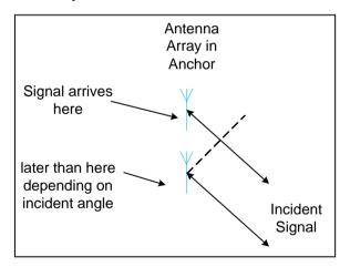
Figure 8: AoA antenna array
