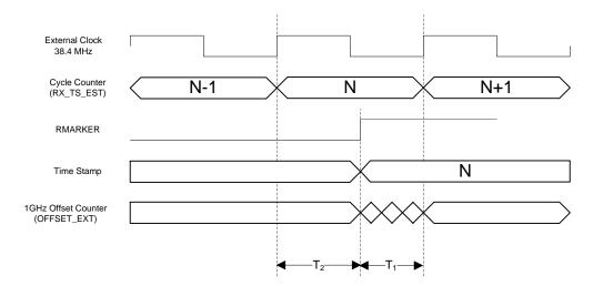
Figure 25: OSRS Mode Receive Timebase Synchronisation
