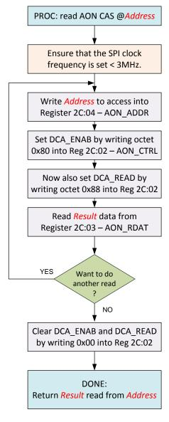
Figure 28: Flow chart for direct read of AON address
