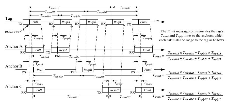
Figure 39: Ranging to 3 anchors with just 5 messages where each anchor calculates its own range result
