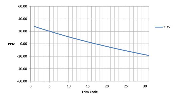
Figure 29: PPM vs Crystal Trim Setting, V<sub>BATT</sub>= 3.3 V
