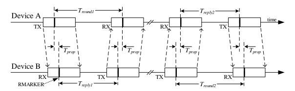
Figure 37: Double-sided two-way ranging with four messages
