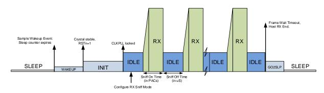
Figure 19: Power profile for SNIFF where a frame is not received
