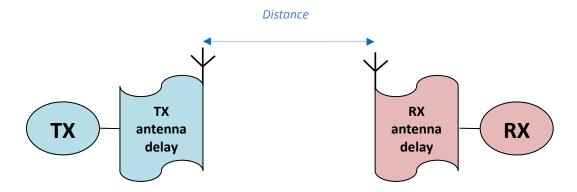
Figure 30: Transmit and Receive Antenna Delay
