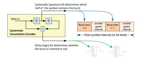
Figure 32:- BPM/BPSK data and PHR modulation
