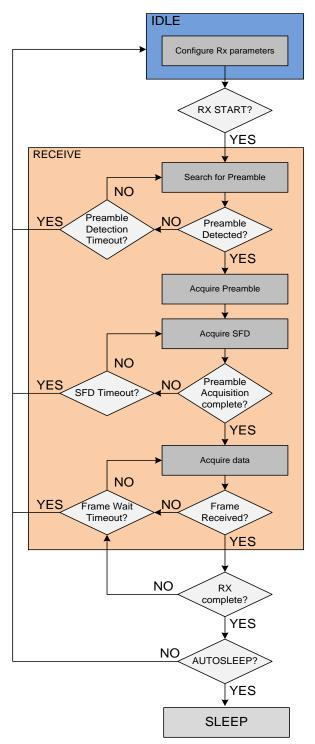
Figure 13: Basic receive sequence
