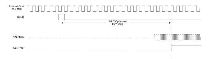
Figure 24: Synchronised Transmission
