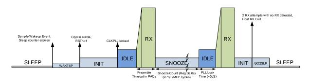
Figure 17: Power profile for low power listening mode where no frame is received
