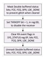
Figure 15: TRXOFF in Double-Buffered Mode
