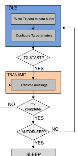
Figure 11: Basic Transmit Sequence
