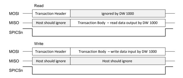
Figure 1: SPI Read and Write Transactions
