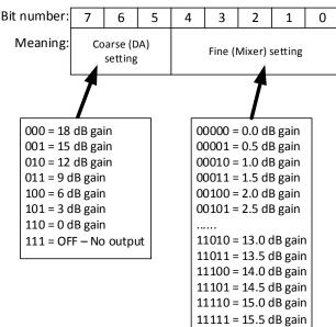
Figure 26: Transmit power control octet
