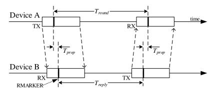
Figure 36: Single-sided Two-way ranging
