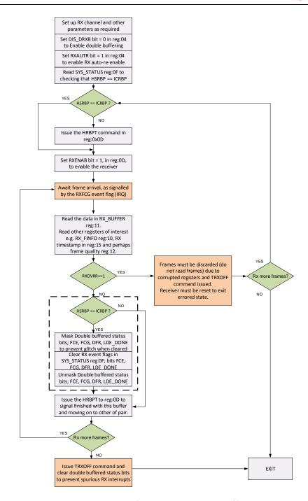
Figure 14: Flow chart for using double RX buffering
