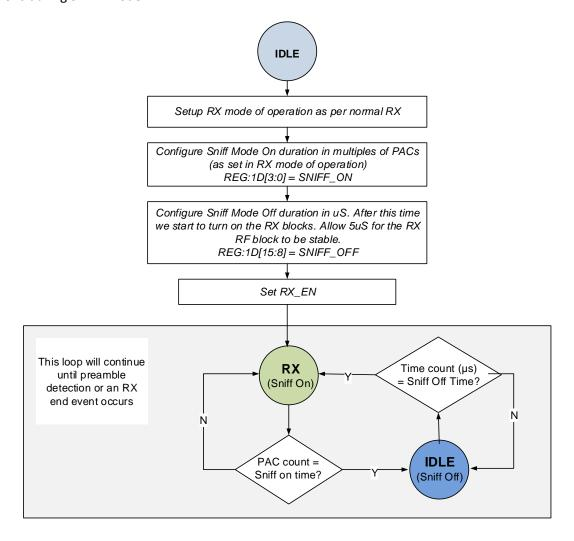
Figure 18: State transitions during SNIFF mode
